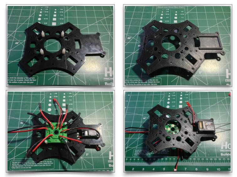
5) Pop 4 vibration dampeners into the APM Plate and affix the APM controller using 3M tape. If you are using another controller such as a KK 2.0 or KK Blackboard use the provided 50x50mm mounting holes. One set mounts at 45 deg. (Blackboard) while the other mounts perpendicularly (KK 2.0). A gimbal controller can also be
