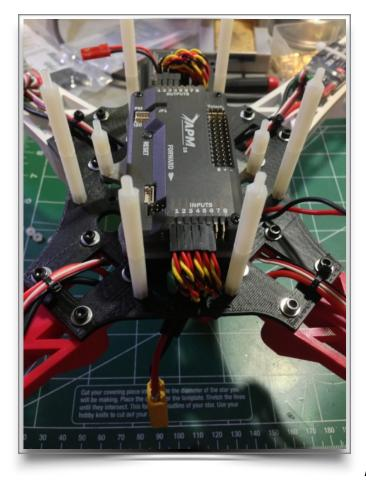
your flight controller and all ESC signal wires to the outputs on your Flight Controller. You could also probably use some of those zip ties to keep things nice here as well.
