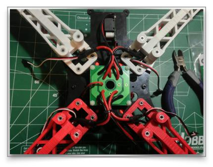
need to be plugged into specific channels on your controller. See the photo below for the APM motor arrangement. Simply take a sharpie marker and draw a 1-4 hash marks near the plug end to identify the wire when plugging them into the flight controller outputs.
