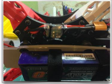
Now that you have the main body and all the electronics installed you should go ahead and measure out the main power lead, cut it to length and solder on a female XT60 connector. Route it through one of the rectangular holes and plug it into the current sensor "out". The only thing left to do is to install the Top Cover. Plug the GPS/ Compass wires into the APM and attach the Top cover to the nylon standoffs with nylon nuts. Again take care not to strip the threads by over torquing.
