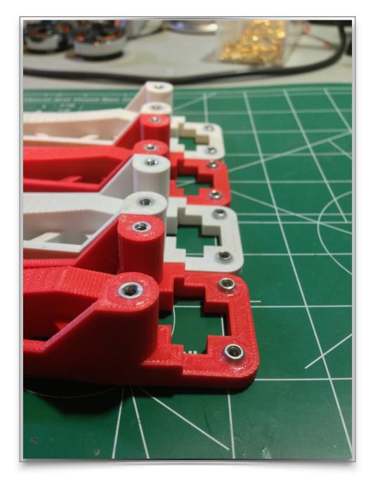
2) Assemble the Top Cover. As I mentioned earlier I am using an APM 2.6, I designed the top cover for the GPS and compass module as well as my video transmitter and FPV camera. Use 3M tape to adhere the video transmitter, GPS/compass module and FPV camera in place. Use zip ties on unused holes to route the camera cable on the bottom of the top cover. Refer to the pictures for which holes to use zip ties on and which holes to leave for the standoffs.
