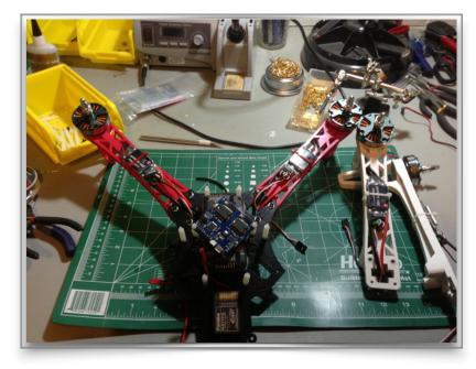
wires into the Power Distribution Board. Black to black, red to red. I know it sounds stupid but double check everything is plugged in correctly. Cross a wire here and you can screw some shit up!
