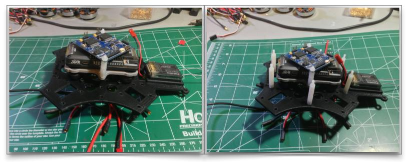
mounted above the APM either at 45 deg. or by using the Gimbal Mount Plate. Mount the APM Plate to the Top Plate with the vibration dampeners. The vibration dampener balls can be very effective at isolating vibrations from the APM. Below is a graph showing measured vibrations that are half of what is acceptable levels with no balancing of the props. Also before you are done with the Top Plate add six nylon
