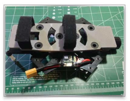
the Battery Tray before securing it to the Bottom Plate. It is also easiest to add all six dampeners to the Battery tray then attach to the Bottom Plate. Also add two standoffs (1<sup>"</sup>) at the aft part of the frame. If you are using metric standoffs you may need to add a couple washers to get the spacing correct. Its also a good idea to route and affix your current sensor if you are
