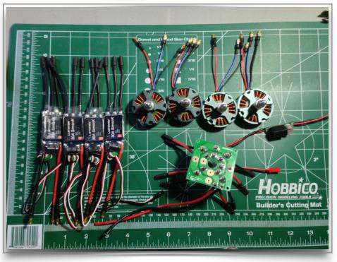
4) Mount the power distribution board to the bottom of the Top Plate using short standoffs, M3 bolts and nylon nuts. Make sure all power leads are oriented the way
