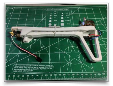
motors to determine which way they need to spin. If they spin the wrong direction just swap any two wires. Affix the ESC to the arm with either 3M or zip ties.
